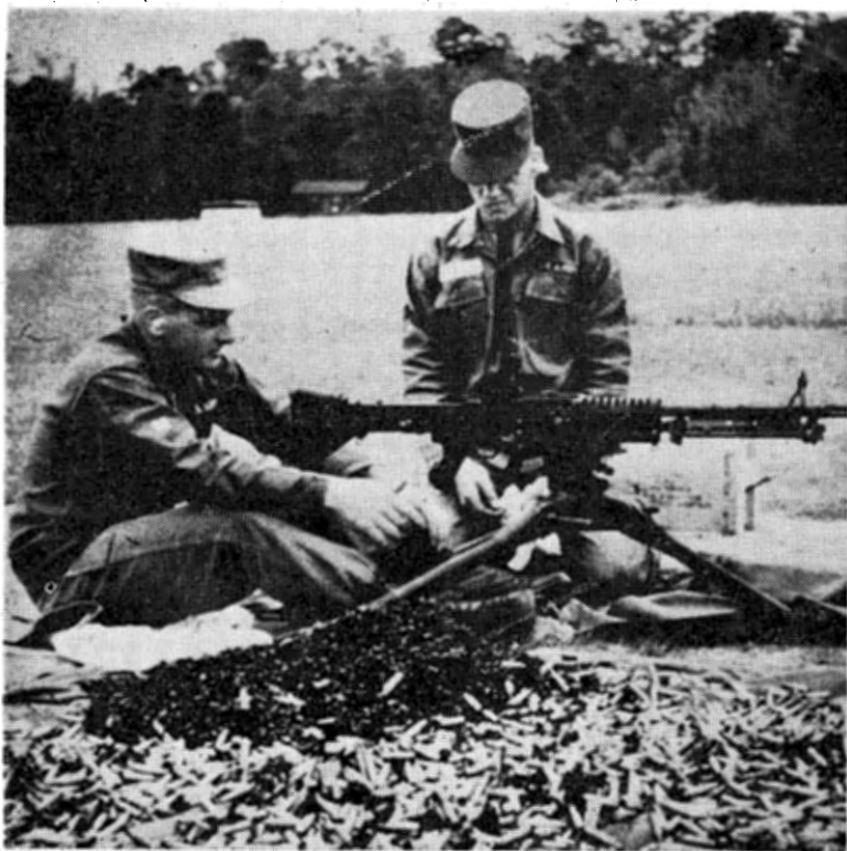
A LOT OF AMMO . . . More than a quarter of a million rounds of ammunition were fired by the Infantry Board during the user test of the new M-60 lightweight general purpose machine gun. Here board members check the durability of the weapon by continuous sustained firing tests.
