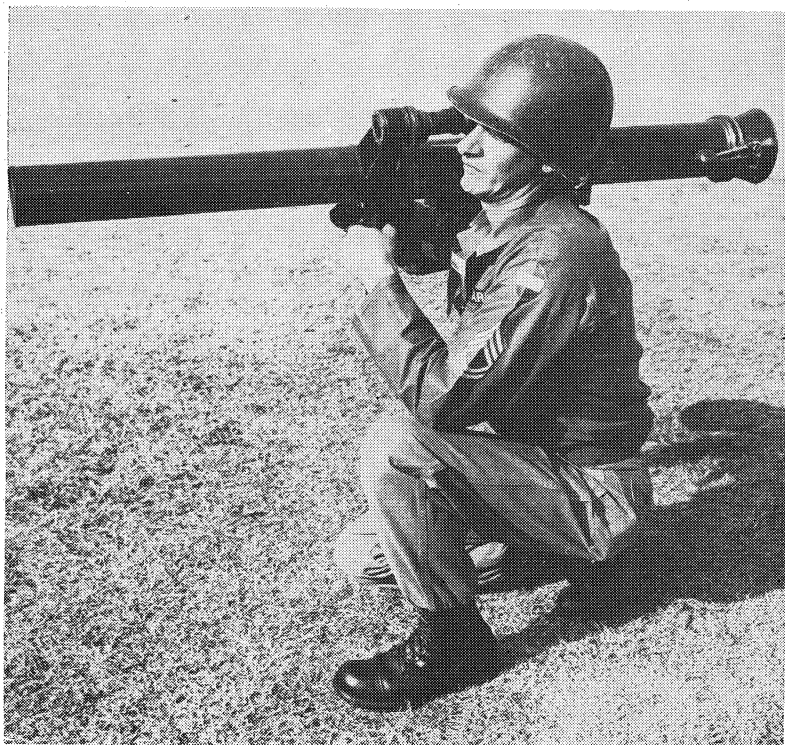
The 90 mm recoilless rifle is a lightweight, man-portable anti-tank weapon that can be fired from the shoulder or from an integral ground mount.
