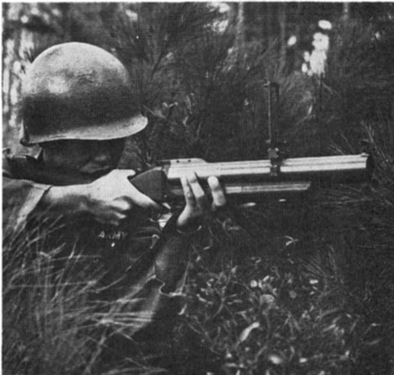
The XM-79, a single shot grenade launcher recently tested by the Board, fires 40 mm rounds with considerable accuracy up to ranges of 400 meters.
