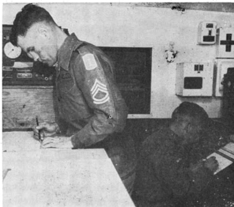
Sfc Floyd Garwood computes wind direction and velocity as the data is received by the control recorder. Behind him Sfc Jerry Russell compiles information on temperature, air pressure and relative humidity as it is received by the radiosonde recorder.
