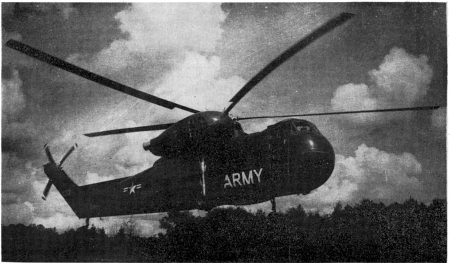
LARGEST ARMY HELICOPTER . . . The H-37, largest helicopter in use in the Army today, has two 2,500 horse power engines. It features a forward clam shell door that opens in the front of the aircraft, facilitating loading and unloading.
