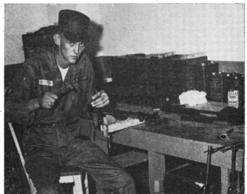
Unit armored Sp4 Richard L. Fortner of Cocoa, Fla., 138th Transportation Company (Light Truck), Florida National Guard unit on active duty here, gets his unit weapons in shape for marksmanship qualification. Here he replaces a rear sight assembly on a .30 caliber U. S. carbine.
