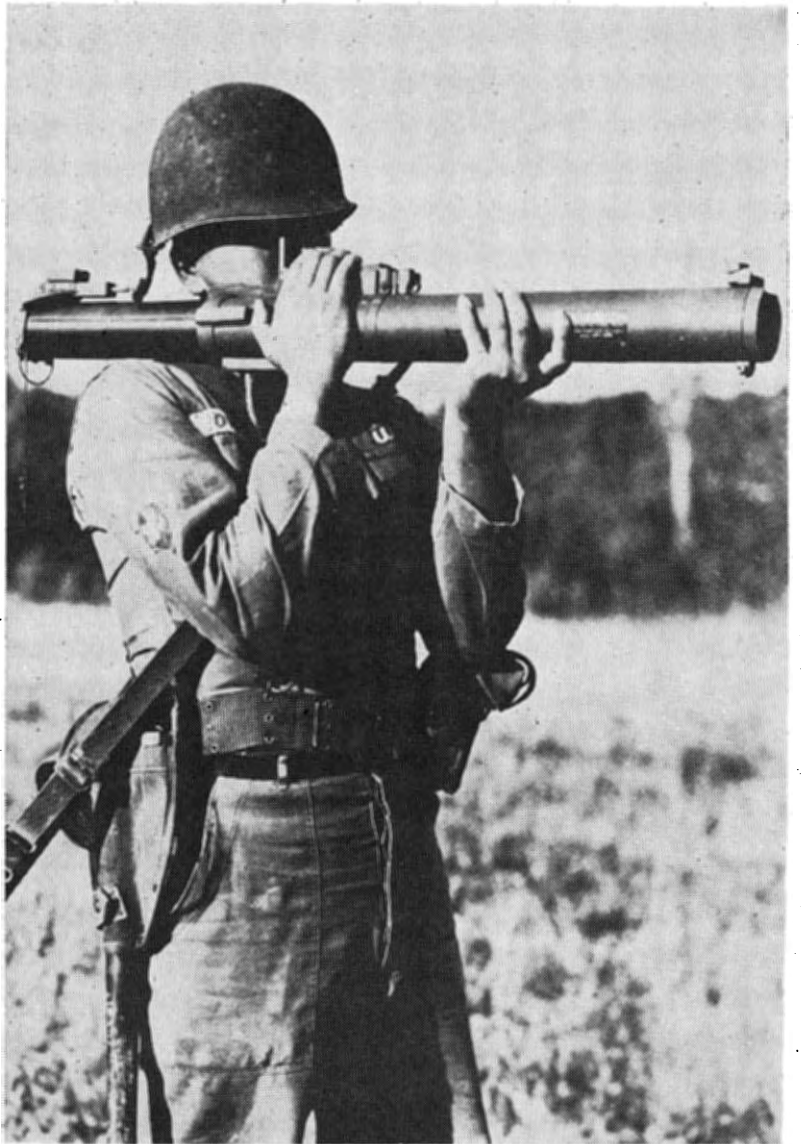
Light anti-tank weapon XM-52 weighs less than five pounds. Carrying case serves also as launcher that can be discarded after firing.
