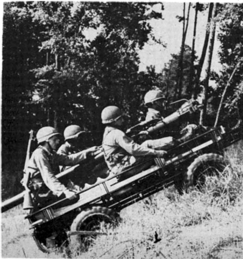
MULES MOVE OUT . . . Helicopter-transported 106mm recoilless rifle and mechanical mule with full crew move into the attack. From the left are Cpl. Phillip L. Callahan, Sgt. Hayward L. Wallace, Sgt. Oscar Miranda, and Sfc Richard Trapier.
