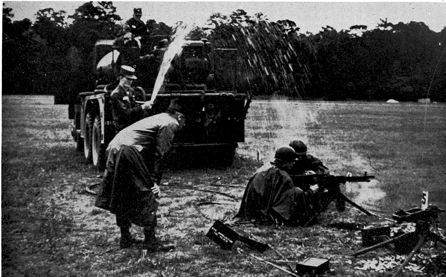
MACHINE GUN TESTS . . . The M-60 lightweight general purpose machine gun underwent severe checks during its user tests conducted by the U.S. Infantry Board. Here board members find that if sunny days appear when rain tests are scheduled, a fire hose will easily replace the nebulous cloud.
