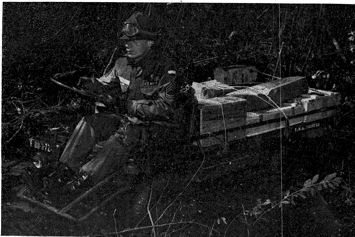
THE ARMY'S NEW MULE . . . The mechanical mule, a four-wheel vehicle designed to relieve the foot soldier of the burden of carrying heavy weapons and equipment in the front line areas, is shown undergoing user tests conducted by the Infantry Board here. Here a board member checks the operation of the vehicle across swampy territory.
