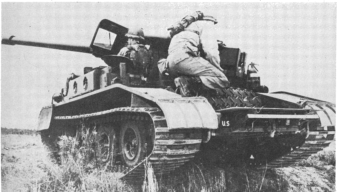
One of the newest combinations in the Infantry arsenal is the full-tracked self-propelled 90-mm gun which is seen during the problem.
