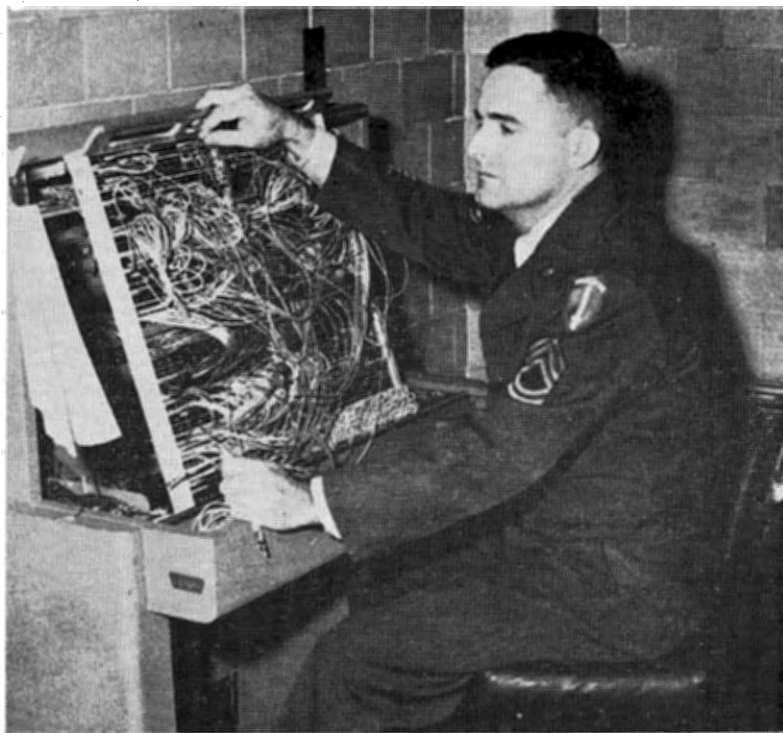
Sfc Kendred Taylor, operates a 407 IBM electrical accounting machine which prints 100 lines per minute, with a performance that is said to equal that of 80 error-free, high-speed typists working at one time.
